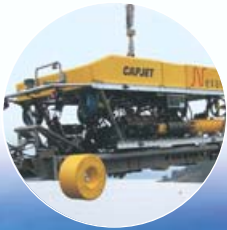
Special laying ships and ROVs for submarine cable laying, trenching and back-filling
